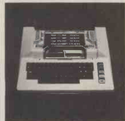
Atari 800 Console (with cover removed)
